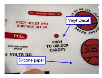
Smaller decals such as propeller decals and service marks will most likely not have any application film.
