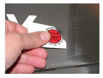
Slowly and carefully pull the silicone sheet away while initially holding the small tab of decal film that has been applied to the surface.
